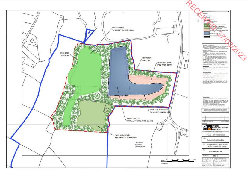
Figure 5-16 Restoration Plan (Hydro Environmental Services, 2022)
